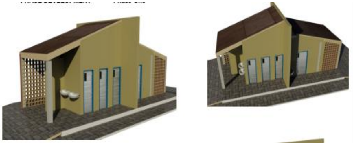
Figure 2: A public toilet with narrow typology constructed at Kemisse to test the developed management model and engineering design: with different side views
